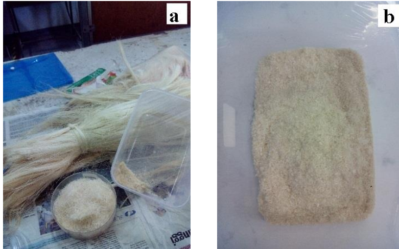
Fig. 1. Pineapple Leaf Fiber (a) original and (b) powdered.
